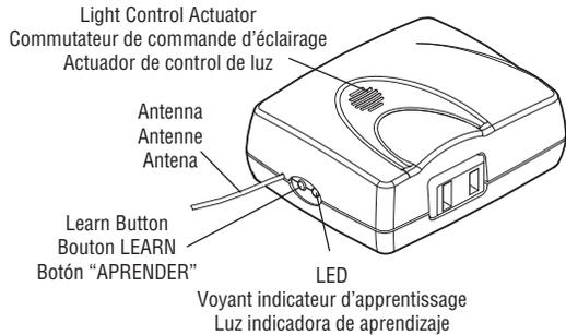
The Security+® Remote Light Control is designed to operate lights according to the rating chart shown. Please read the instructions and power limitations carefully to ensure proper use and maximum safety. NOT recommended for use with toasters, coffee pots, florescent or halogen lighting systems. **Use 120 Vac polarized outlet only.**
